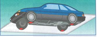
slows the rotation of the tires. They react against the pavement slowing the vehicle.
